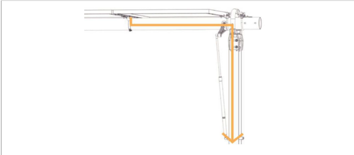
Figure 2-2: Grounding path for PV modules
